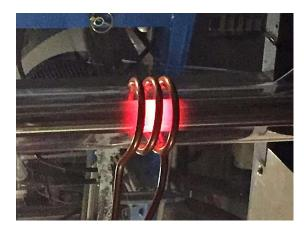
NanoH<sup>TM</sup> system shown in use to coat metals on the interior of metal tubes.
