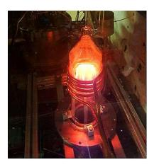
NanoV<sup>TM</sup> system shown in use to grow high resistance (undoped) and n-type doped Ga2O3 epi.
